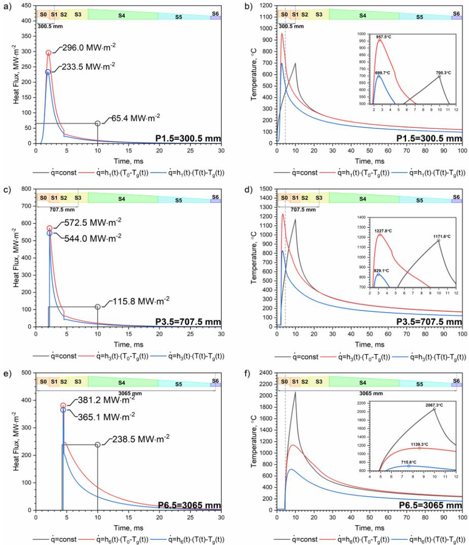
Fig. 6. Different approximations of the relation  $\dot{q}_i(t, r_{in}, z)$  in the 3 zones S1, S3, and S6 – left side of the figure. The temperature distribution  $T_i(t, r_{in}, z)$  of the barrel's inner surface at the same zones – right side of the figure.
