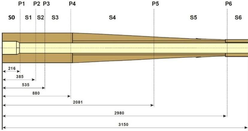
Fig. 1. Heat transfer zones S1 to S6 of the 35 mm cannon barrel input to the calculations: S1: 0÷385 mm,  $r_{out} = 55.0-55.0$  mm; S2: 385÷535 mm,  $r_{out} = 55.0-57.0$  mm; S3: 535÷880 mm,  $r_{out} = 57.0-59.5$  mm; S4: 880÷2081 mm,  $r_{out} = 59.5-44.07$  mm; S5: 2081÷2980 mm,  $r_{out} = 44.07-31.0$  mm; S6: 2980÷3150 mm,  $r_{out} = 31.0$  mm.
