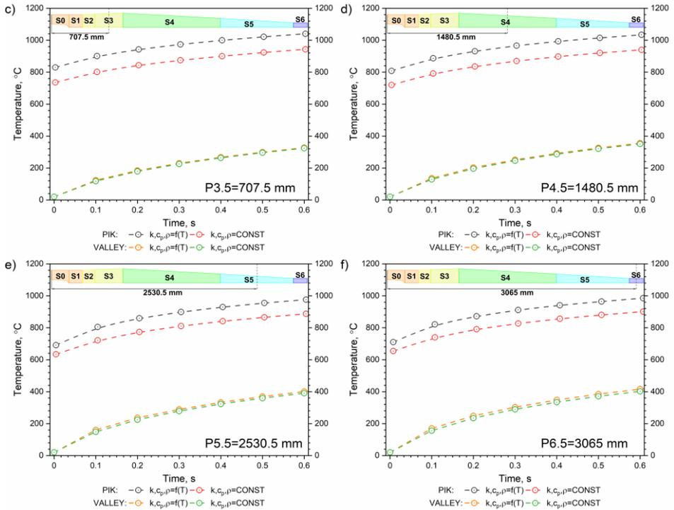
Fig. 5. Envelope of the lowest and the highest temperatures of the inner surface at the 6 zones S1 to S6 for the sequence of seven shots, for the thermophysical properties of variable as a function of temperature, i.e.,  $k, c_p, \rho = f(T)$  [2] and for the thermophysical properties of constant, i.e.,  $k, c_p, \rho = \text{const}$ .
