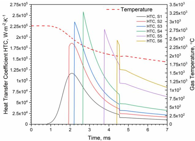
Fig. 2. Heat transfer coefficient (HTC) as a function of the time  $h_i(t)$  in the 6 cross-sections P1 to P6 and the gas temperature as a function of the time  $T_g(t)$  for the 35 mm anti-aircraft cannon barrel [2].
