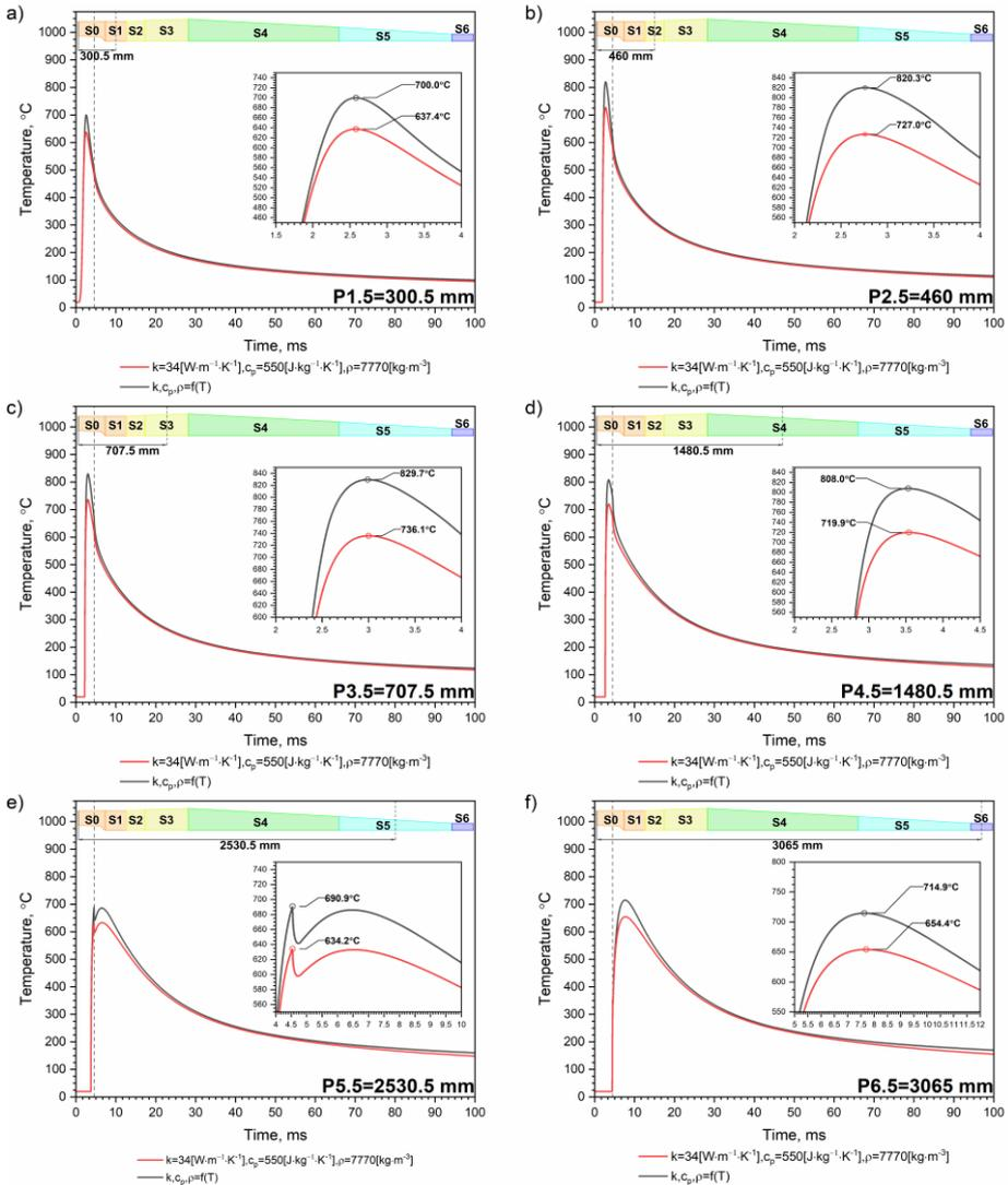
Fig. 3. The temperature distribution  $T_i(t, r_{in}, z)$  of the barrel's inner surface at the 6 zones S1 to S6 for a single shot for the thermophysical properties of constant and variable as a function of temperature
