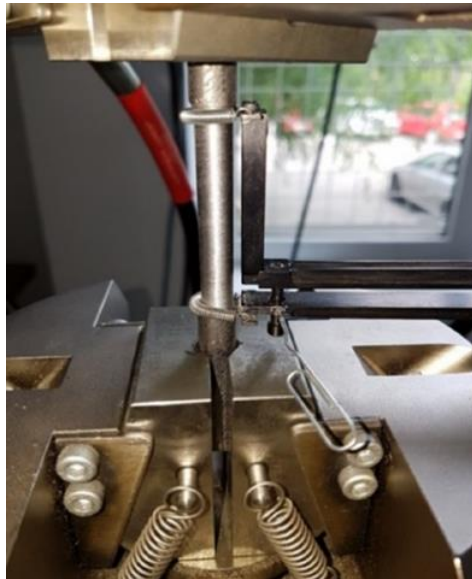
Fig. 2. A cylindrical sample mounted in a universal testing machine's clamp [2]
