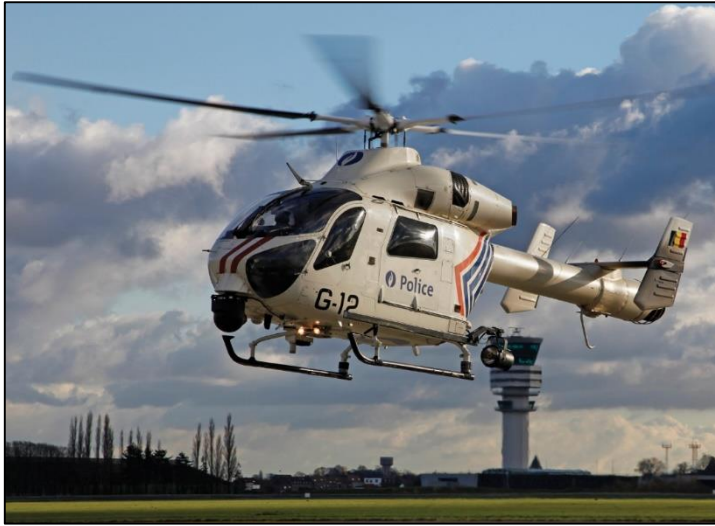
Fig. 10. MD-902 Explorer utility helicopter with NOTAR system 13
