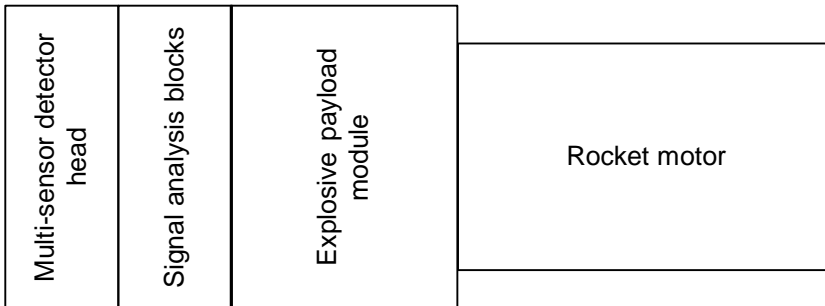
Fig. 2.1. Concept of the general counter-projectile structure
