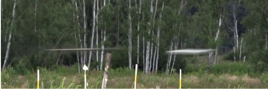
Fig. 4.1. Automatically launched counter-projectile (see right) and the armour-piercing projectile (see left) in flight (on an intercept course)
