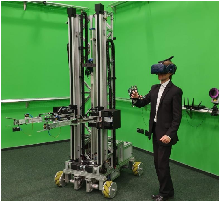
Fig. 1. Two-armed, mobile, remotely controlled robot implementing telepresence concepts
