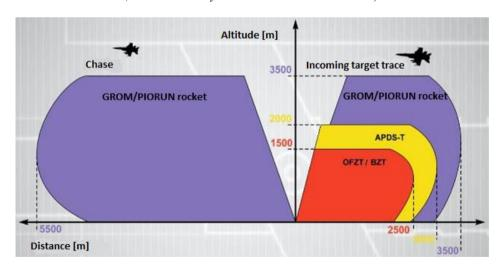
Fig. 2. PILICA's target elimination capabilities: APDS-T - a subcalibre anti-tank missile, OFZT - a cluster-demolition-ignition-track missile, BZT - an ignition-track anti-tank missile
