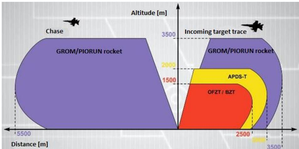
Fig. 2. PILICA's target elimination capabilities: APDS-T - a subcalibre anti-tank missile, OFZT - a cluster-demolition-ignition-track missile, BZT - an ignition-track anti-tank missile
