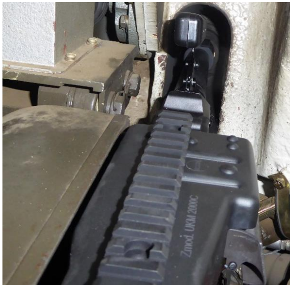
Fig. 5. Modified UKM 2000C mounted in the tower of a PT-91 tank
