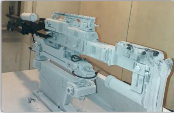
Fig. 3. Modified UKM 2000P – low-temperature testing
