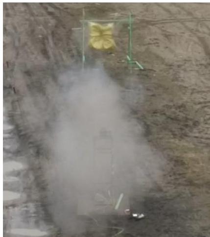
Image 4. Experimental short-range rocket missile shown hitting the target's aramid-fibre curtain. Image captured by the VIS light video camera of the DJI Inspire Pro drone
