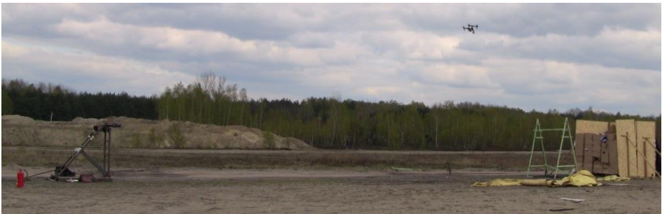
Image 3. Live firing range test stand during its setting up, comprising the launcher of the experimental short-range rocket missiles (see left), the target trap cantilever (see right) with the aramid-fibre curtain laid next to it and optionally backed with a stack of cardboard boxes, as recorded by the DJI Inspire Pro drone hovering overhead
