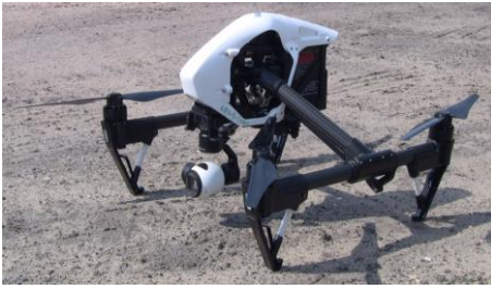
Image 1. DJI Inspire Pro visual observation drone with a VIS light video camera onboard
