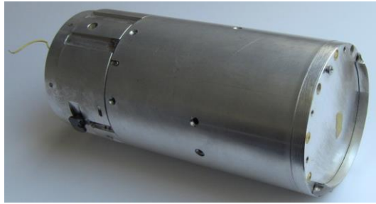
Image 8. Inertial guidance head, containing the flight recorder, traced by the Bielik drone operator (note the slight damage to the head's casing)
