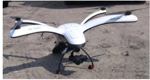
Image 2. Bielik visual observation drone with an IR video camera onboard
