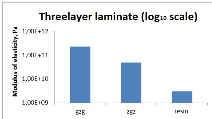
Fig. 6. Calculated values of the modulus of elasticity for the three-layer laminate specimen models
