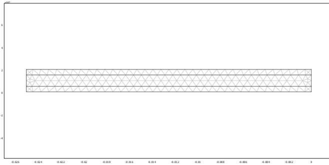
Fig. 2. Diagram of the three-layer laminate specimen breakdown into finite triangular elements
