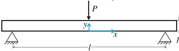
Fig. 1. Diagram of loading the test specimen (a beam) with a force input applied in between the supports
