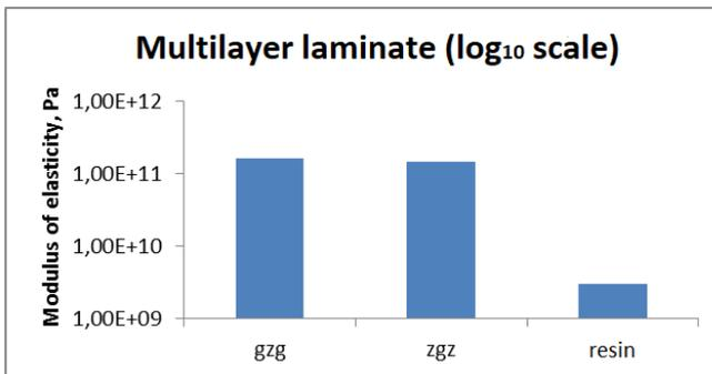
Fig. 5. Calculated values of the modulus of elasticity for the multi-layer laminate specimen models
