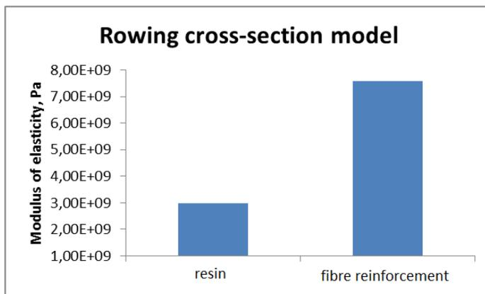
Fig. 7. Calculated values of the modulus of elasticity for the rowing cross-section model in the transverse configuration
