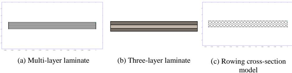
Fig. 3. Models of the specimen internal structure types
