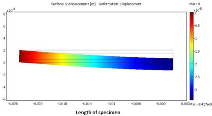
Fig. 4. Examples of the numerical simulation results produced for the three-layer laminate specimen in the  $gzg$  configuration: distribution of displacements along the axis  $Oy$ , with a presentation of the outline of the deformed specimen
