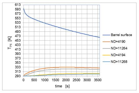
Fig. 19. Charts of temperature changes as a function of time in selected points of the cover in profile P6 for the second boundary condition variant
