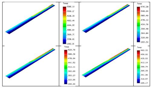
Fig. 15. Temperature field distributions in the horizontal profile of the barrel-barrel cover assembly at times t = 60 s, 600 s, 1800 s, 3600 s from installing the cover (temperatures given in K)
