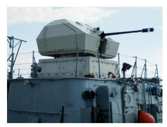
Fig. 1. 35 mm automatic naval gun installed on ORP Kaszub
