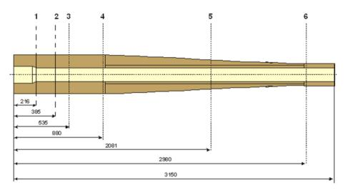
Fig. 5. Longitudinal profile of the gun barrel with indicated calculation profiles and external radii  $r_z$  of the barrel wall.
