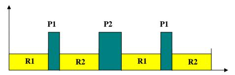
Fig. 20. Firing cycle for standard munitions and kinetic energy penetrators: R1 – rhythm 1, R2 – rhythm 2; P1 – pause 180 seconds; P2 – pause 600 seconds
