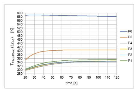
Fig. 7. Temperature changes on the external barrel surface at subsequent profiles from P1 to P6, during the period from time 20 s to 120 s
