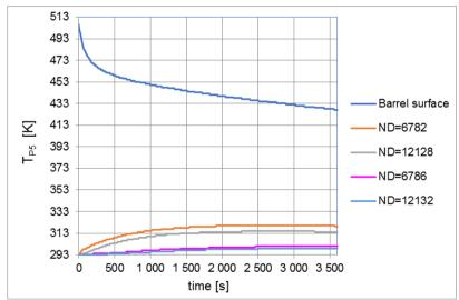
Fig. 17. Charts of temperature changes as a function of time in selected points of the cover in profile P5
