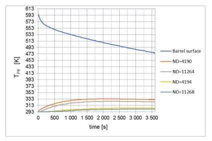
Fig. 16. Charts of temperature changes as a function of time in selected points of the cover in profile P6
