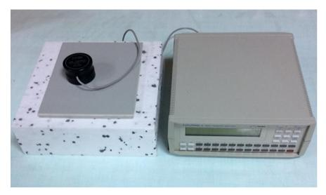
Fig. 11. Test station for testing thermophysical properties of the gun barrel cover composite material using the Isomet 2104 instrument and the API 210412 surface probe (at room temperature)
