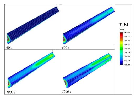
Fig. 18. Temperature field distribution on the external surface of the barrel cover at times t = 60 s, 600 s, 1800 s, 3600 s from installing the cover (second variant of boundary conditions). For time t = 3600 s, a temperature distribution on the bottom surface of the cover is also shown
