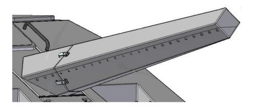
Fig. 4. View of gun section with barrel cover installed
