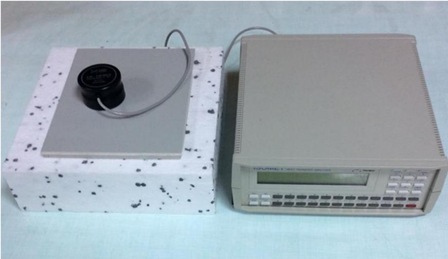
Fig. 11. Test station for testing thermophysical properties of the gun barrel cover composite material using the Isomet 2104 instrument and the API 210412 surface probe (at room temperature)
