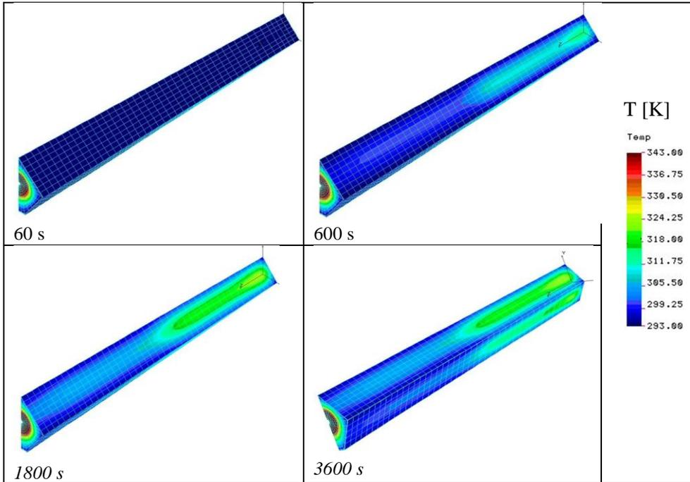
Fig. 18. Temperature field distribution on the external surface of the barrel cover at times  $t = 60$  s, 600 s, 1800 s, 3600 s from installing the cover (second variant of boundary conditions). For time  $t = 3600$  s, a temperature distribution on the bottom surface of the cover is also shown
