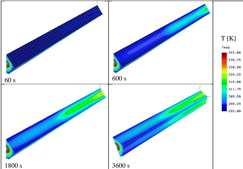
Fig. 14. Temperature field distribution on the external surface of the barrel cover at times  $t = 60$  s, 600 s, 1800 s, 3600 s from installing the cover. For time  $t = 3600$  s, a temperature distribution on the bottom surface of the cover is also shown
