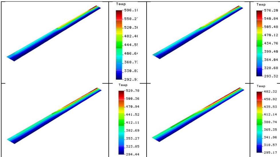
Fig. 15. Temperature field distributions in the horizontal profile of the barrel-barrel cover assembly at times  $t = 60$  s, 600 s, 1800 s, 3600 s from installing the cover (temperatures given in K)
