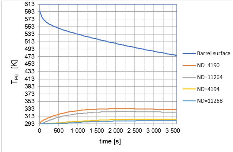
Fig. 16. Charts of temperature changes as a function of time in selected points of the cover in profile P6
