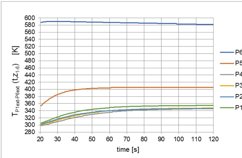
Fig. 7. Temperature changes on the external barrel surface at subsequent profiles from P1 to P6, during the period from time 20 s to 120 s
