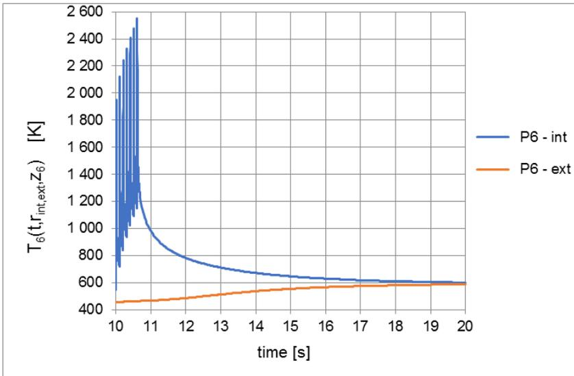
Fig. 6. Temperature changes on the internal (blue) and external (brown) barrel surfaces for the most heavily loaded profile P6 after the third seven-shot burst
