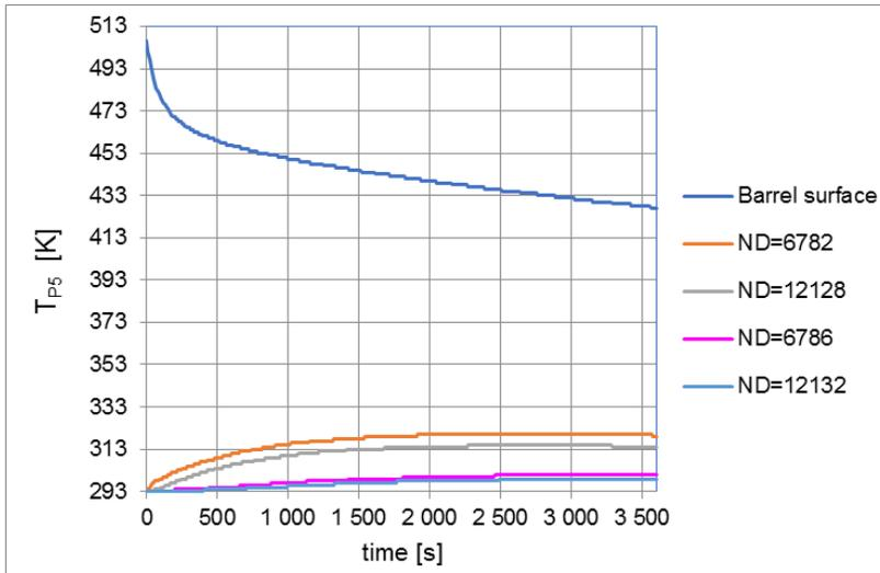
Fig. 17. Charts of temperature changes as a function of time in selected points of the cover in profile P5
