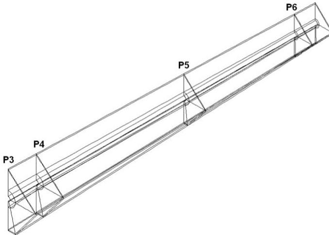
Fig. 9. Profiles P3-P6 of the barrel-cover assembly, adopted for the initial condition problem and the boundary conditions
