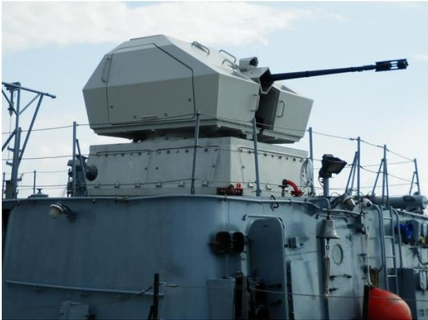
Fig. 1. 35 mm automatic naval gun installed on ORP Kaszub
