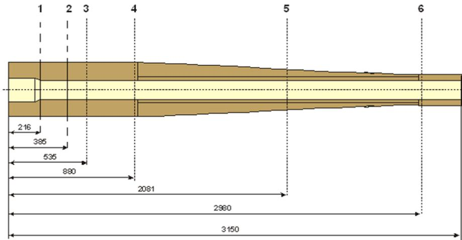
Fig. 5. Longitudinal profile of the gun barrel with indicated calculation profiles and external radii  $r_z$  of the barrel wall.
