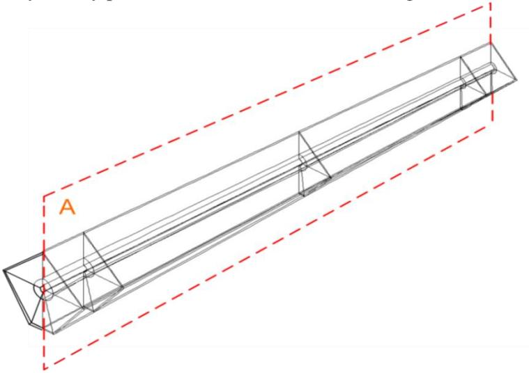
Fig. 8. Division of the entire barrel-cover assembly volume into two parts with a vertical symmetry plane running along the barrel axis
