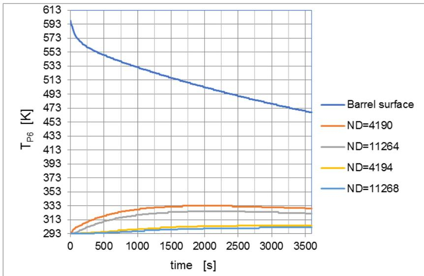
Fig. 19. Charts of temperature changes as a function of time in selected points of the cover in profile P6 for the second boundary condition variant
