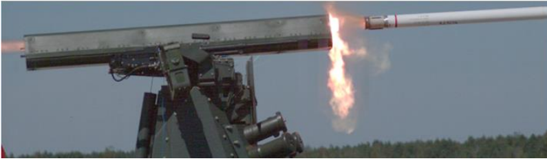
Fig. 9. Impact of exhausted gases on the launcher (from t_4 = 81.144 ms to t_6 = 125.244 ms)
