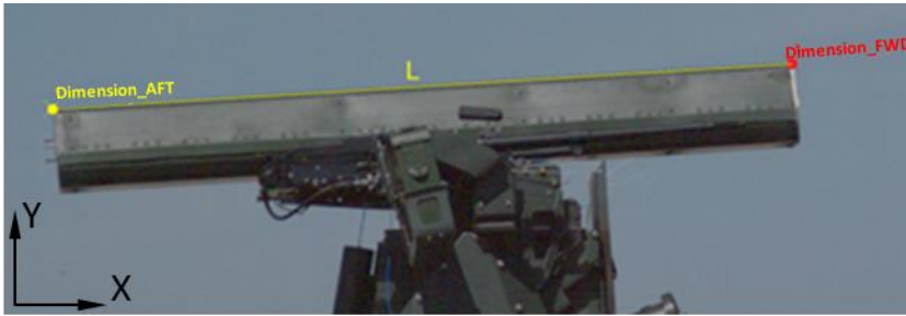
Fig. 12. Dimension of the launcher length (L) with the denoted reference points in TEMA Motion program
