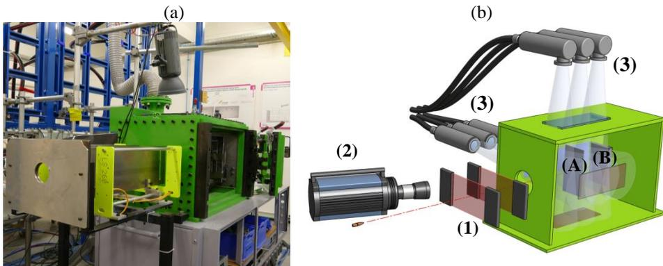
Fig. 3. Experimental set-up (a), and its schema (b): (A) perforated plate, (B) Mars<sup>®</sup> 190, (1) dual-light barrier, (2) ultra-high speed camera, (3) triple flash X-radiography
