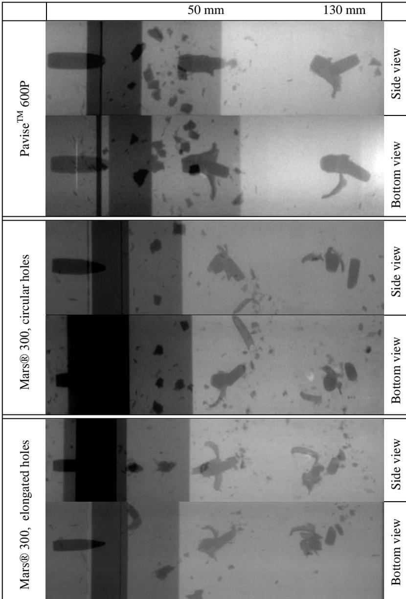
Fig. 7. Flash X-ray images of the projectiles which hit in the ligaments between the holes
