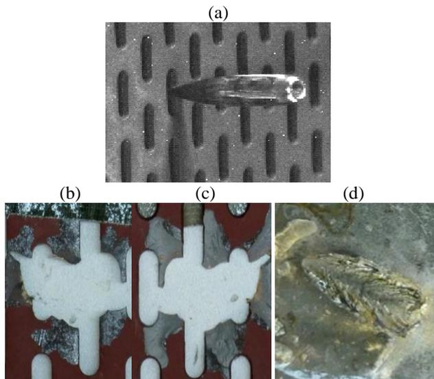
Fig. 5. Projectile hit in a hole of the bainitic perforated plate: a) impact position. Damage mode of the pre-armor plate: (b) front face, (c) rear face and (d) deformation of the main armour
