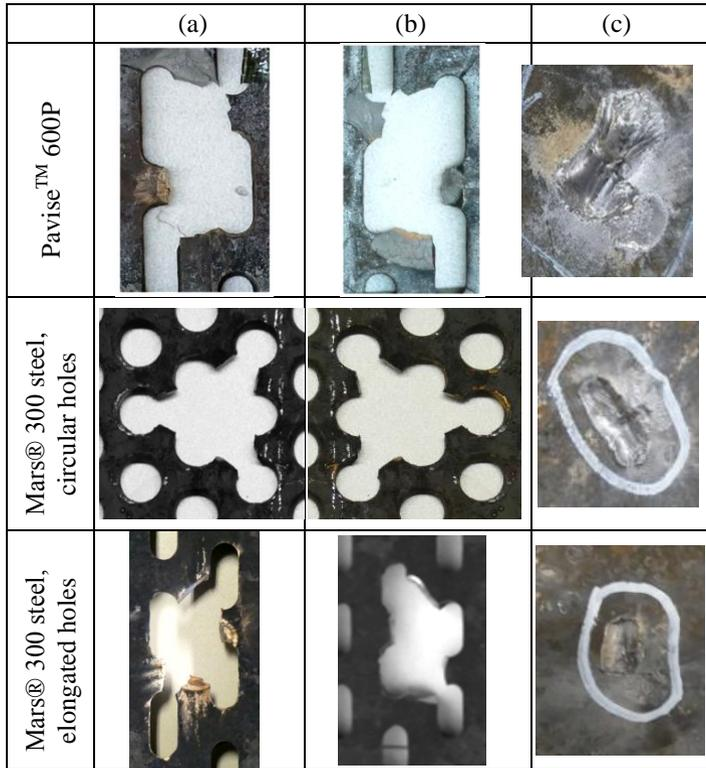
Fig.8. Damage modes resulting from the impacts in ligaments. Perforated plates: (a) front face and (b) rear face. (c) Damage of the main armour
