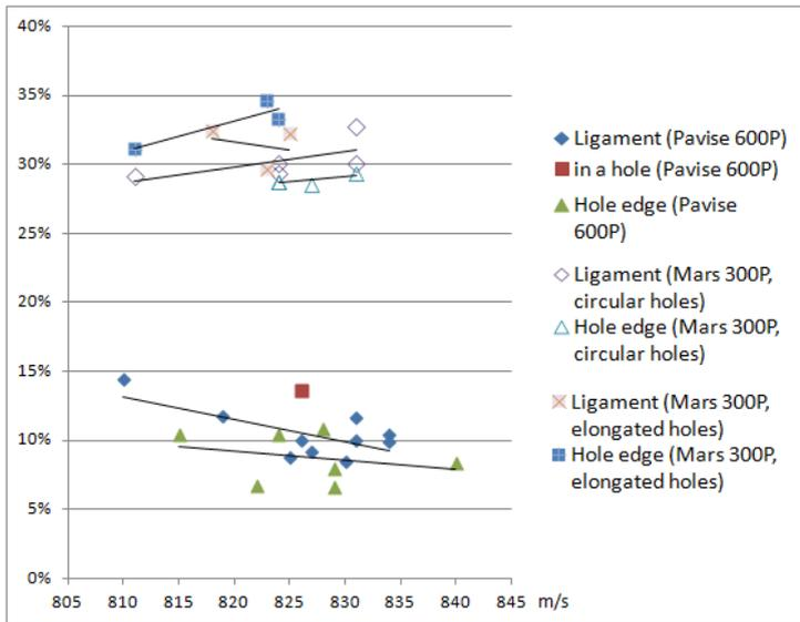
Fig. 4. Decrease in the bullets impact velocity
