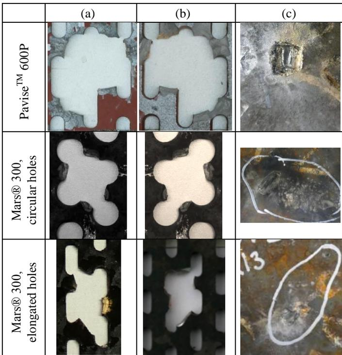
Fig. 10. Damage modes resulted from the impacts at a hole-edge. Perforated plates: (a) front and (b) rear face. (c) Damage of the main armour
