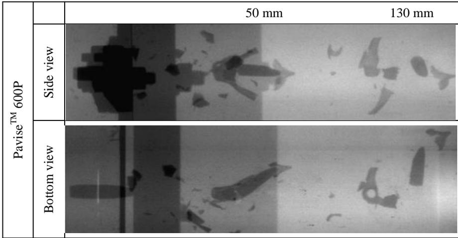
Fig. 6. Flash X-ray images of the trajectory of the bullet which hit in the hole center
