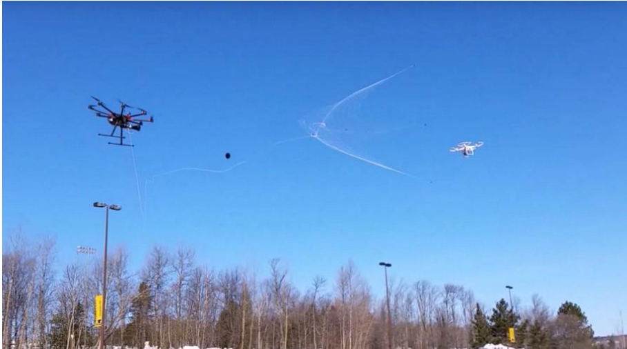
Fig. 5. Counter-UAV built at the Michigan Tech University
