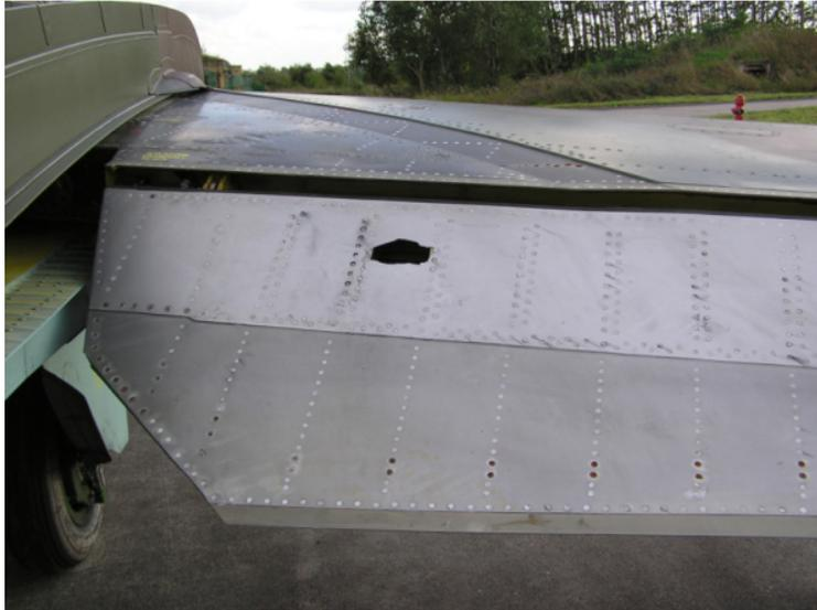
Fig. 2. Damage to a Su-22 flap
