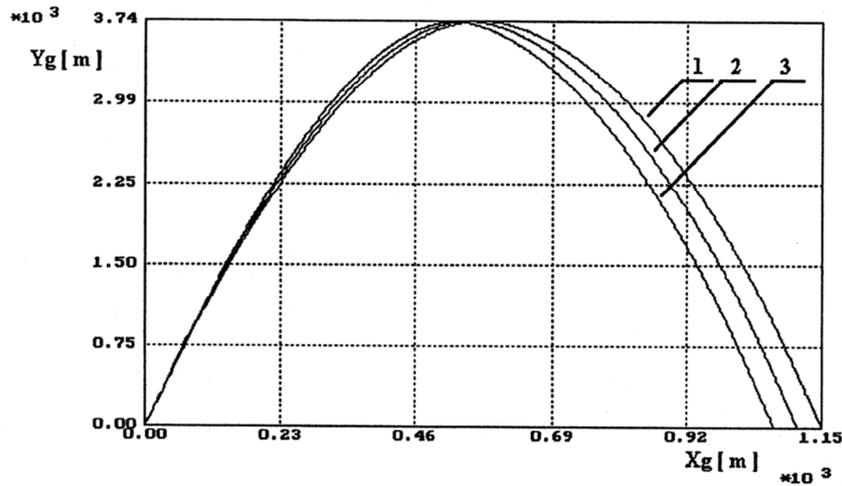
Fig. 8. Relationship  $Y_g = f(X_g)$  for angle of elevation  $\Theta_0 = 85 [^\circ]$  at the moment of firing, the initial projectile velocity  $V_0 = 320 [m/s]$  and the head wind: 1 –  $W_x = 0 [m/s]$ ; 2 –  $W_x = -5 [m/s]$ ; 3 –  $W_x = -10 [m/s]$
