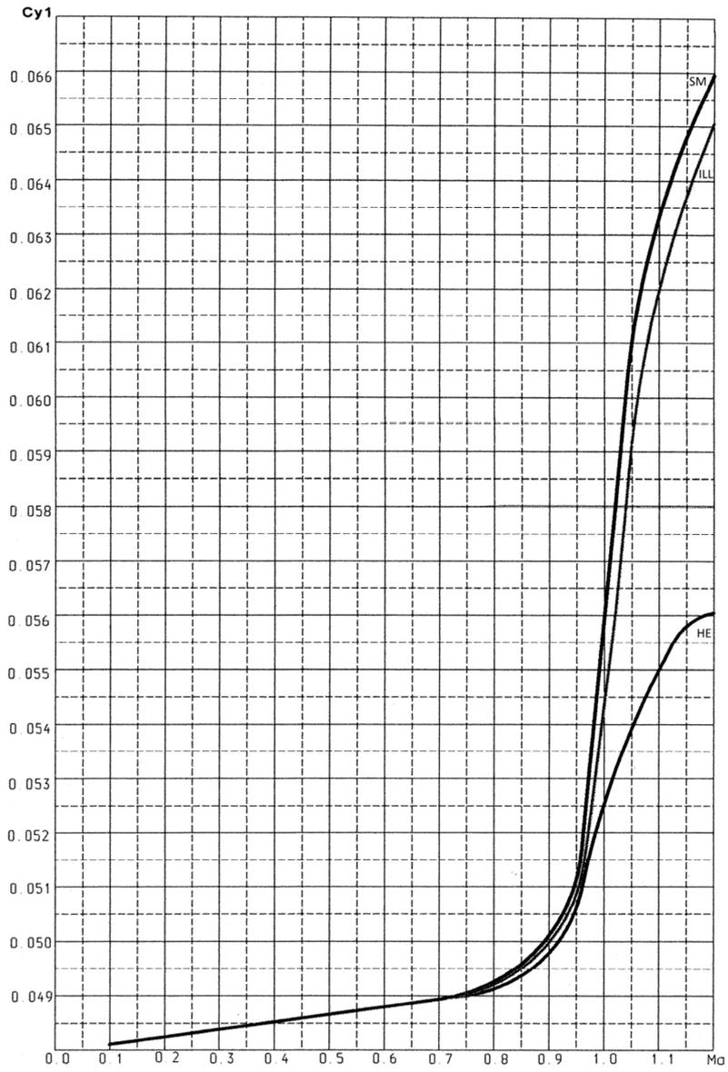
Fig. 3. Projectile lift coefficient in a coordinate system related to the projectile and referenced to the cross sectional area vs. Mach number
