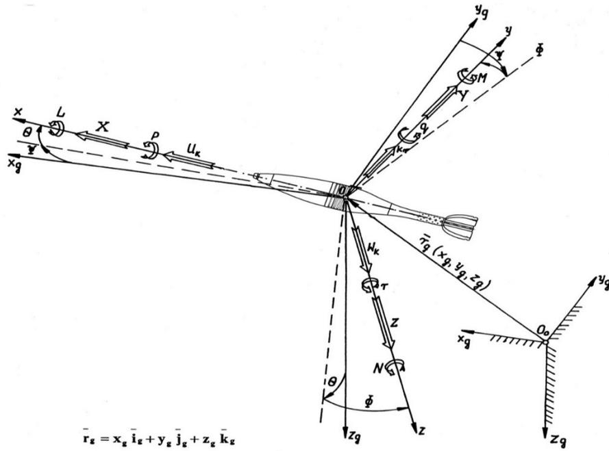
Fig. 5. Assumed linear coordinates  $x_g, y_g, z_g$ ; angular coordinates  $\Psi, \Theta, \Phi$ , coordinate rates of change  $u, v, w, p, q, r$ ; components of the forces and moments of the external forces acting on the projectile in the coordinate system related to the projectile  $0xyz$  [4, 5]
