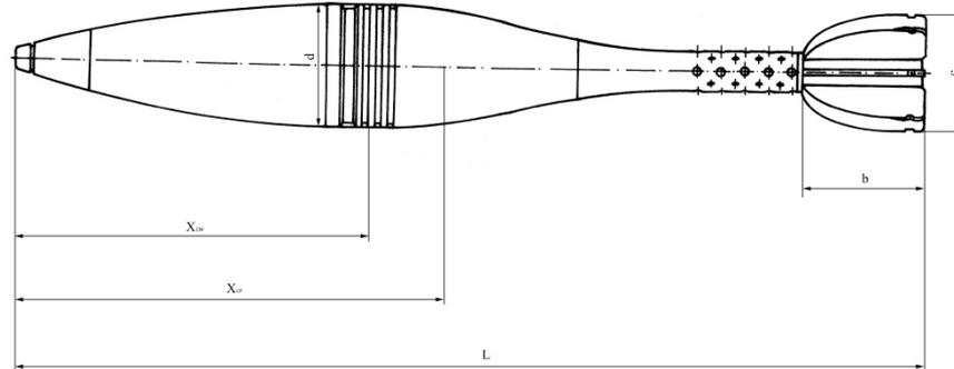
Fig. 1. Aerodynamic model and essential geometric characteristics of the examined mortar shell
