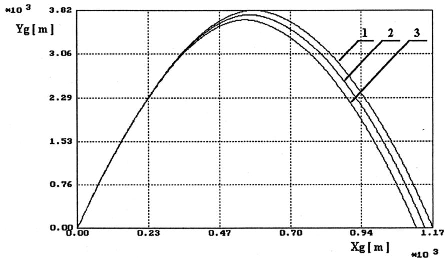
Fig. 7. Graph of the  $Y_g = f(X_g)$  for angle of elevation  $\theta_0 = 85$  [°], velocity  $V_0 = 320$  [m/s] and temperatures: 1 -  $t = t_{\text{nom}} + 15$  [°C]; 2 -  $t = t_{\text{nom}} = 0$  [°C]; 3 -  $t = t_{\text{nom}} - 15$  [°C]
