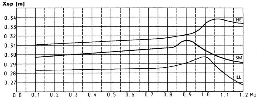
Fig. 4. Centre of the aerodynamic pressure relative to the projectile tip vs. Mach number
