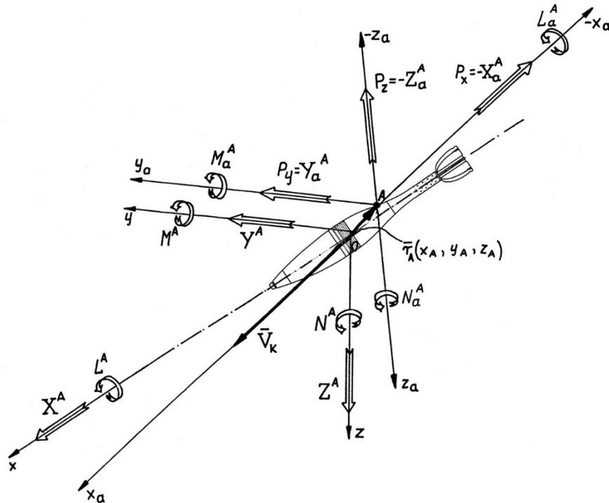
Fig. 6. Forces and moments of the aerodynamic forces acting on the projectile in flight, ref. PN-83 [4, 5]
