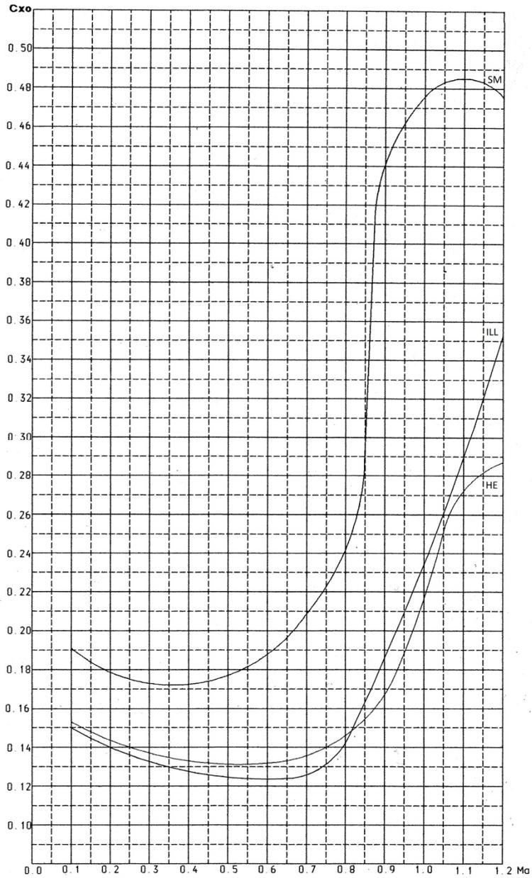
Fig. 2. Drag coefficient  $C_{x0}$  when angle of attack  $\alpha$  is zero, referenced to the cross sectional area vs. Mach number
